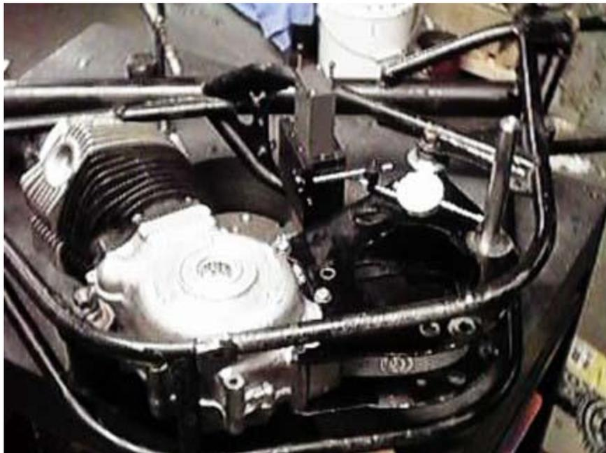
Ken's idea is that if a motorcycle frame isn't right, bending it may get it close, but the only way to get the critical relationship between the steering head and the swing arm pivot right is to measure everything, determine the error, and then re-machine as necessary to correct things. He has learned that taking the easier route of "getting things close" usually means you get to do it over again anyway.
