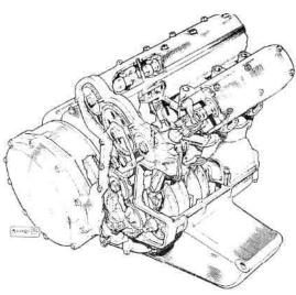
was designed for liquid cooling there was no necessity for the exhaust ports to face forward, and they are, in fact, at the back. Four seperate forward-facing carburetters are specified, although one imagines that they would not benefit from being supplied with warm air from the radiator immediately in front of them:
