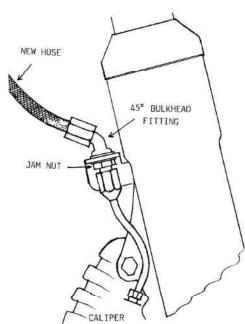
Installation of the hose is pretty straightforward, although you'll find that the black plastic coated securing clips that attach to the upper fork leg are too big for the new hose. I used a piece of black neoprene sheet to take up the slack in the clips so that the hose wouldn't chafe the clips during fork movement.
